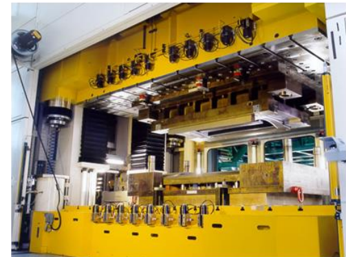
16 000 kN hydraulic Tryoutpress
