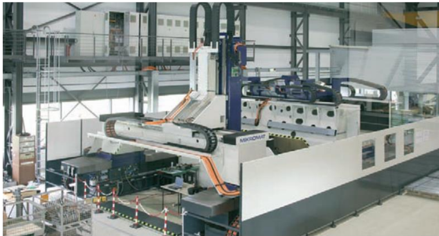
Universal machining centre Dynapod of the IWU
